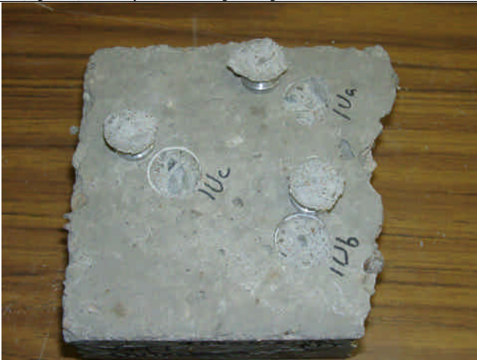
Figure 1 04080003 View of sample 1 (degreased) after dolly adhesion testing showing cohesive failure of the concrete substrate.
