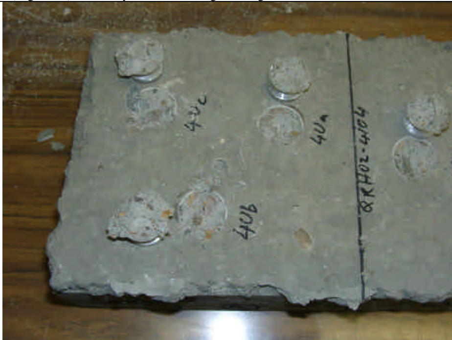
Figure 7 04080029 View of sample 4 (degreased) after dolly adhesion testing showing cohesive failure of the concrete substrate.
