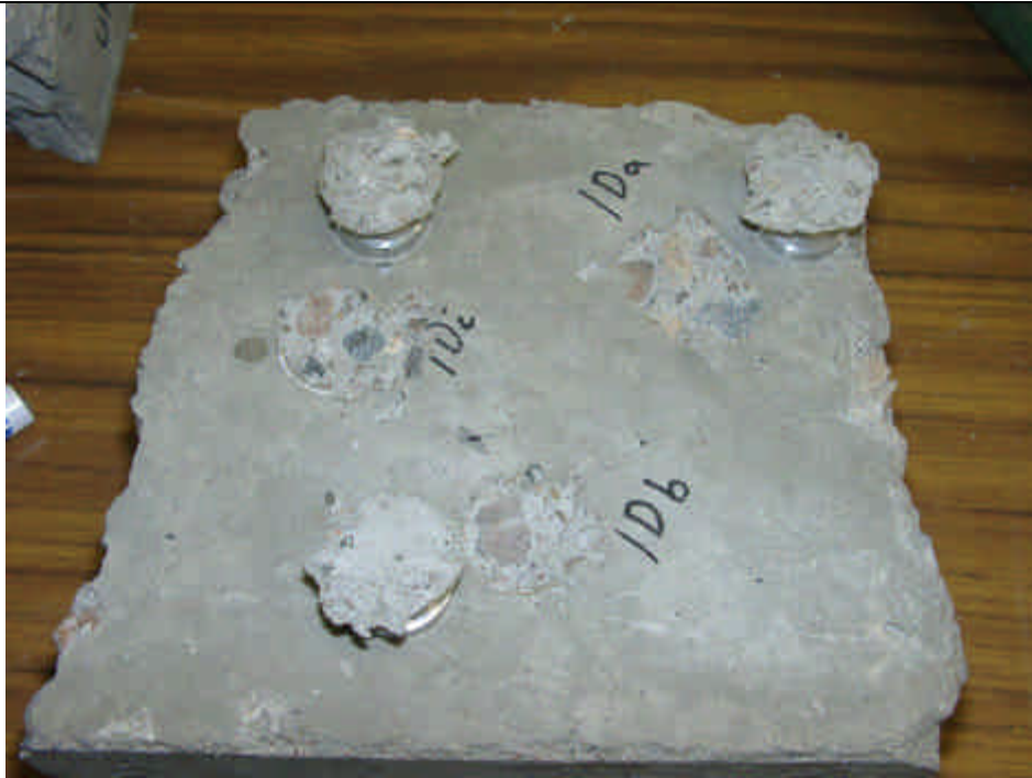
Figure 1 04080003 View of sample 1 (degreased) after dolly adhesion testing showing cohesive failure of the concrete substrate.
