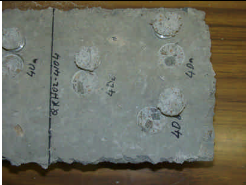
Figure 7 04080029 View of sample 4 (degreased) after dolly adhesion testing showing cohesive failure of the concrete substrate.
